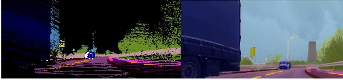
Fig.1 Erroneous semantic class of point cloud projection
